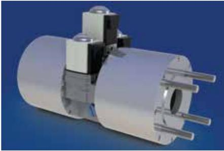
The STEPCON® System is an option to the basic GTI Bi-Fuel® System. STEPCON retains all of the components of the basic fumigation system with the addition of a Gas Control Manifold (GCM), kW sensor, and a panel upgrade with customized firmware and outputs.
