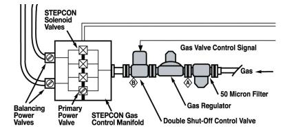
The STEPCON<sup>®</sup> enhances the bi-fuel system, allowing its application over a wider load range, adjusting the optimal substitution rate based on load with the capability to make substitution level adjustments in response to rapid load changes.
