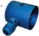
robbing throttle plate. The low restriction air-gas mixer ensures that adequate air-flow is maintained to the engine and that operating efficiencies are not compromised by installation of the device. The computer-aided-design mixer is built to aerospace tolerances using CNC machining processes and is assembled using state-of-the-art welding techniques. The finished mixer has no moving parts and once installed in the
